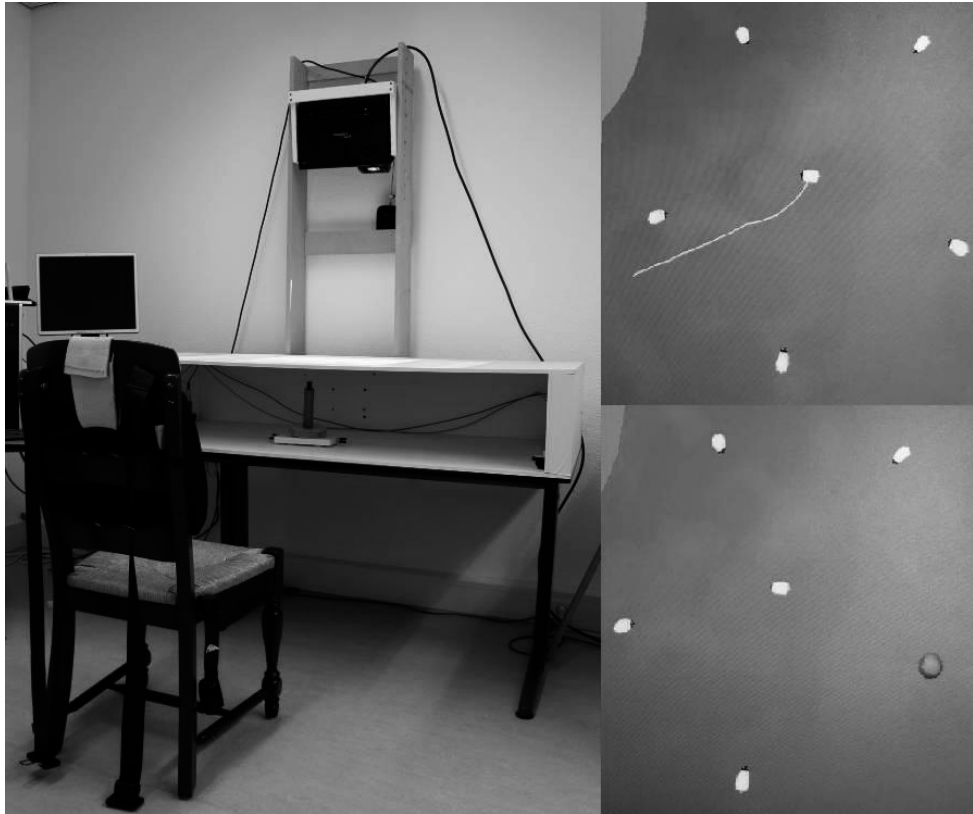
Figure 4.1: Overview of experimental setup. Subjects sat behind the in height adjustable table. They held a hand grip through which hand position was measured. The vision of the arm and hand is obstructed, and a representation of the hand is visualized on the shelf above the arm, projected by a beamer. A representation of the KP and KR feedback, with the five targets and the midpoint of the circle are visualized.
