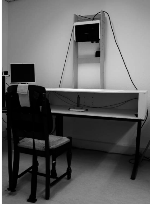
Figure 6.1: Overview of the experimental set-up. Subjects sat behind the in height adjustable table. They held a hand grip through which hand position was measured. The vision of the arm and hand is obstructed, and a representation of the hand is visualized on the shelf above the arm, projected by a beamer.
